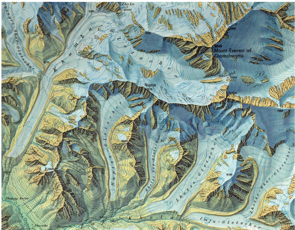
Figure 6: Imhof Map of Everest with manual shaded relief and rock art drawing style – 1962
